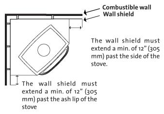
Must be 1" off the wall and 1" off the floor. With standard legs, the shield must be 40" high. With optional short legs, the shield must be 38" high. Both shields must extend and join in the corner.
